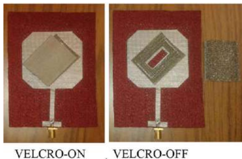
Figure 5: The effective way of using conductive hook and loop to interchange a textile slot patch antenna [15]
