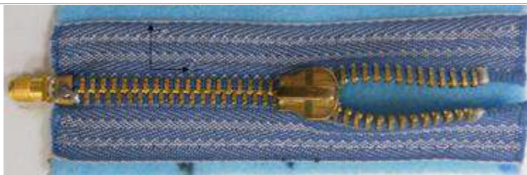
Figure 8: Zip as an antenna [23]
