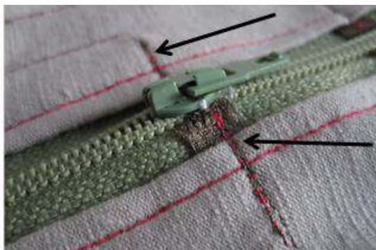
Figure 7: Switching via zip via conductive threads (arrows) [20,21]
