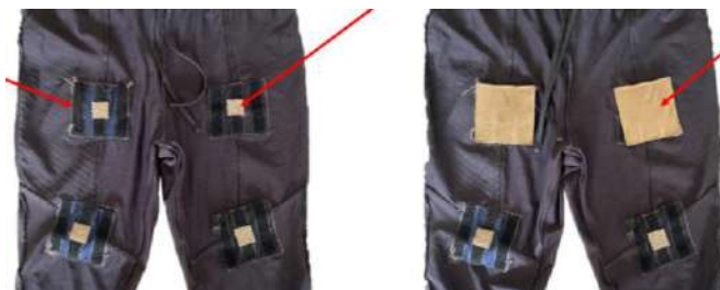
Figure 6: Conductive hook and loop connecting the electrode to the outside of the pants [17]
