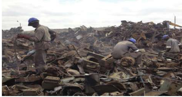
Figure 1 Scrap iron used as a batch in the steel production process from secondary raw materials [13]
