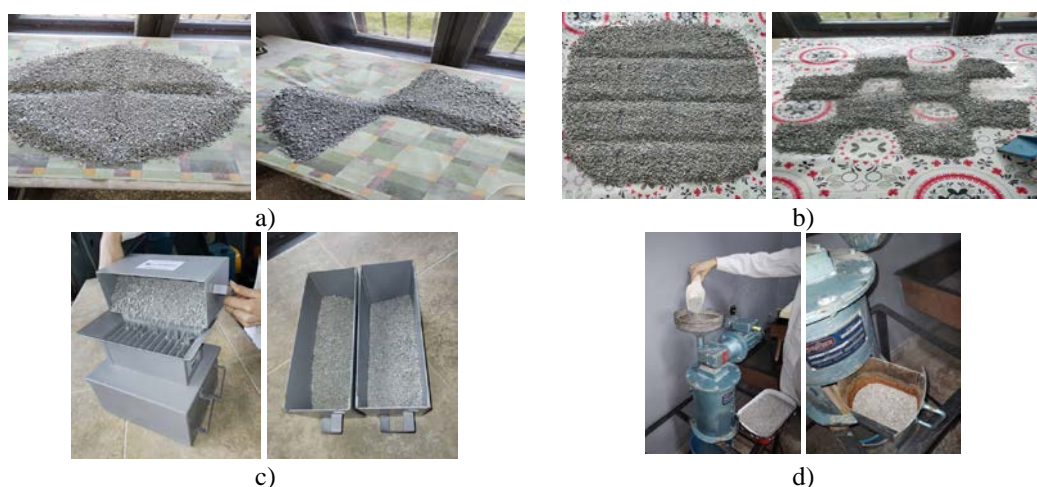
Figure 1 - Applied methods for sample cutting: a) quartering; b) "chessboard" method; c) Jones riffle splitter; d) automatic sampler "Veziin"
