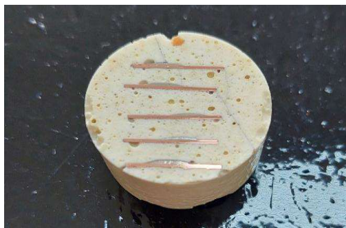
Cured samples prepared for the contact angle measurement.
