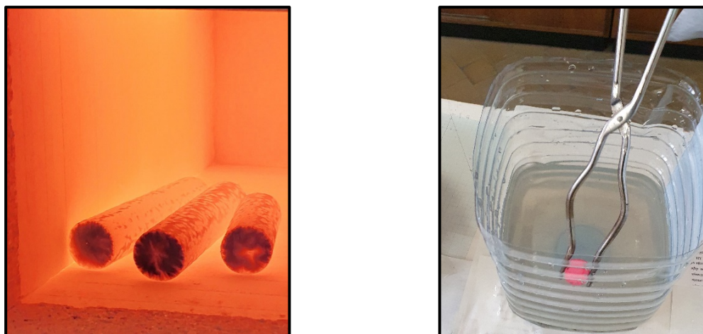
Figure 1 - Heat treatment of steel samples in an electric resistance furnace, followed by quenching
