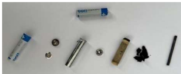
Figure 1 Zn-C batteries and their individual parts
