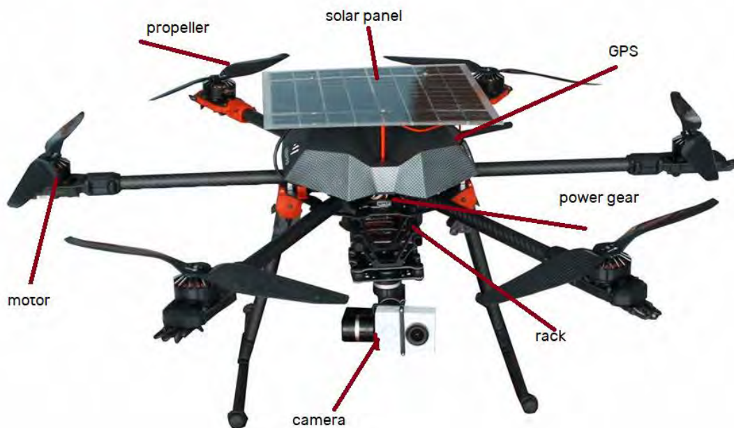
Figure 2. Drone with solar panel
