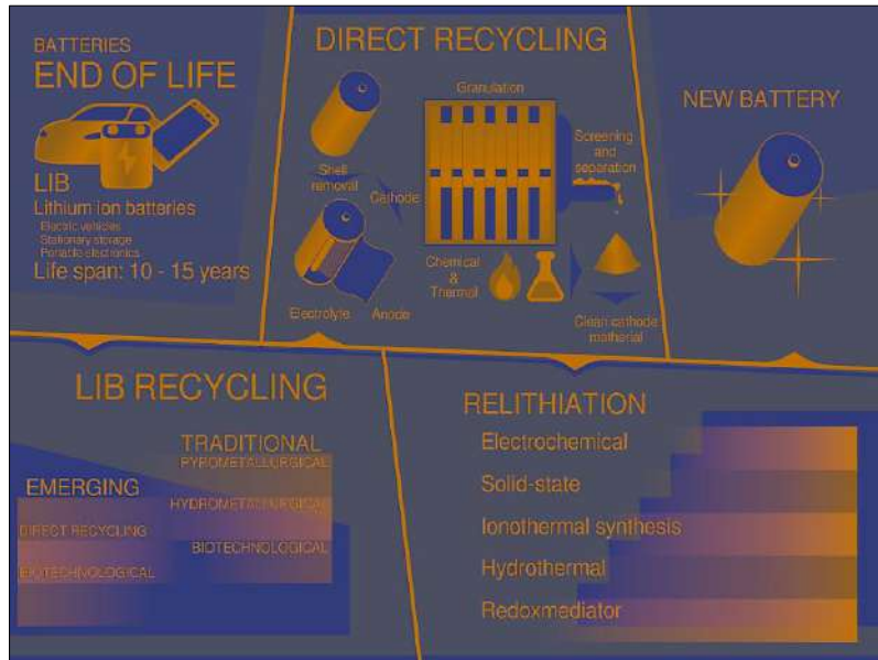
Figure 1 Overview of lithium-ion battery recycling processes: from EOL management to direct recycling and relithiation techniques
